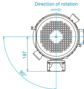
There are upper and lower mounting positions on the pump. Select either one in accordance with the depth of your tank.
