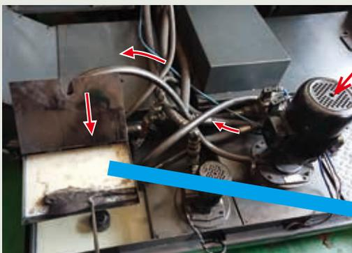
The large flow low pressure unit is discharging sludge.
