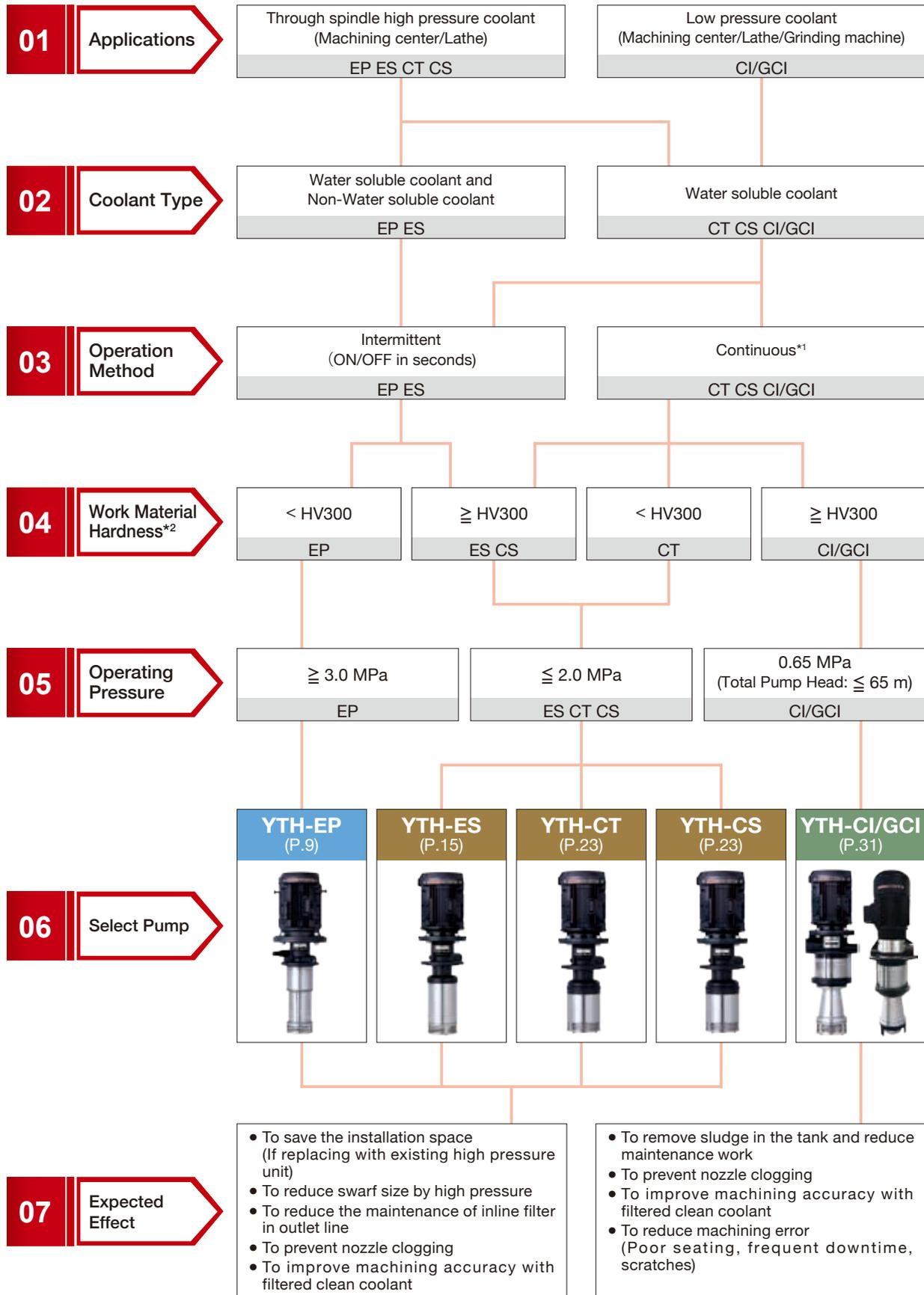
\*1 Intermittent operation is also possible if an unloading valve is installed.
