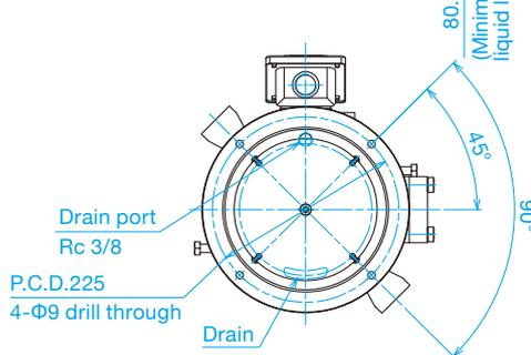
\*If mounting the pump at lower position, be sure to do proper drain piping.
